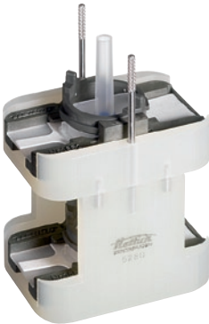
two-tier adapter 5280 illustrated with slide carriers with fastening ring 1662 and cyto chambers 1663
